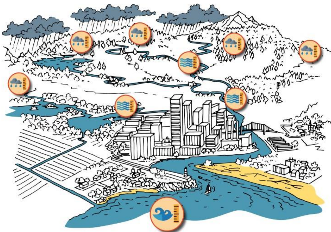
Figure 10_SDAL - Schematic illustration of a watershed instrumented for measuring rainfall, water levels in rivers and streams, and sea level.
